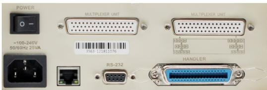
The HT3563 and CHT3563A multi-channel resistance tester can be used for both single-channel test and multi-channel test; They support single-card 12-channel in four-terminal test and max of 24-channel test
