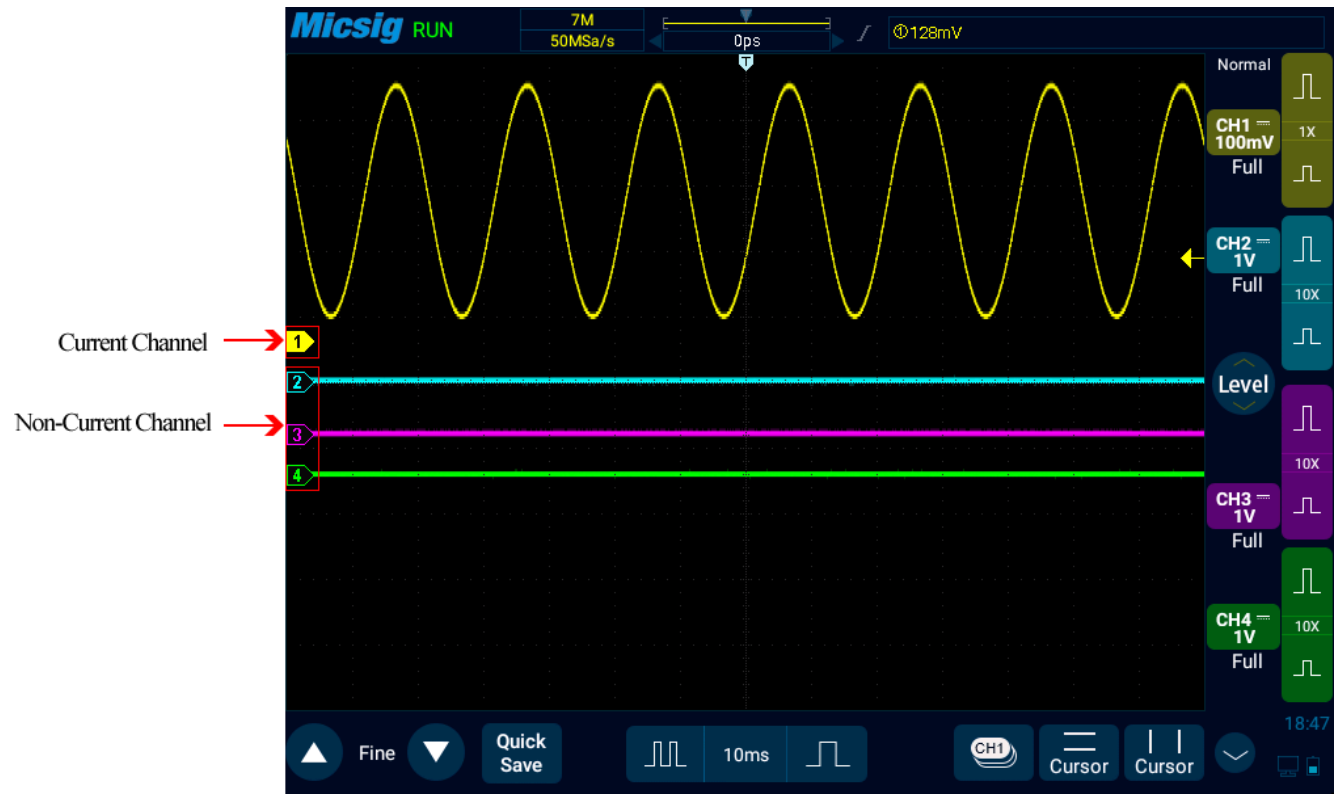
Figure 5-2 Current Channel and Non-Current Channel
