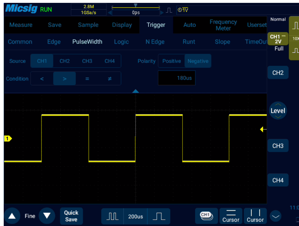
Figure 6-14 Negative Polarity Pulse Level Flip
