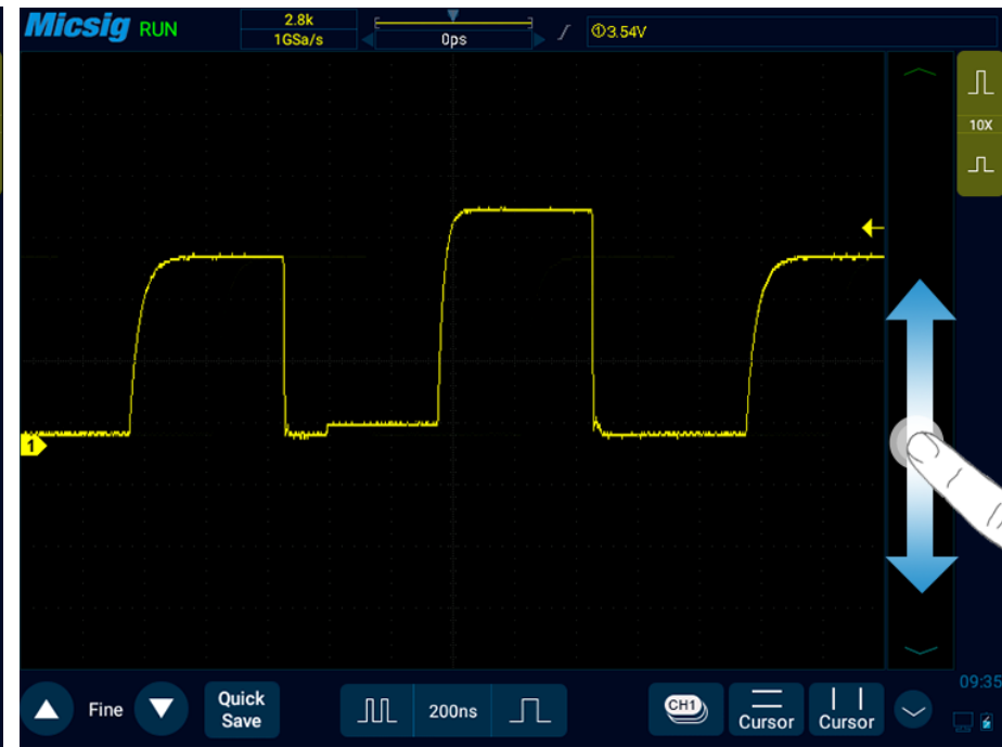
Figure 6-4 Abnormal Signal Captured by Setting Trigger Level
