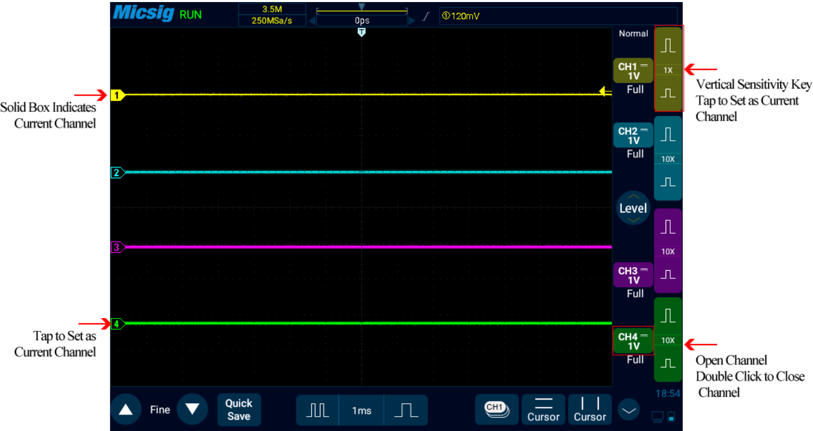
Figure 5-4 Channel Open, Close and Switching
