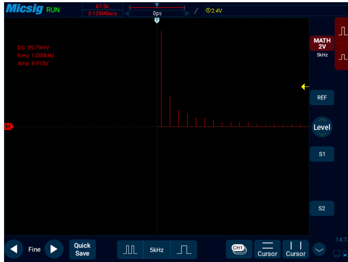
Figure 9-4 Spectrum Amplitude as V-Hz
