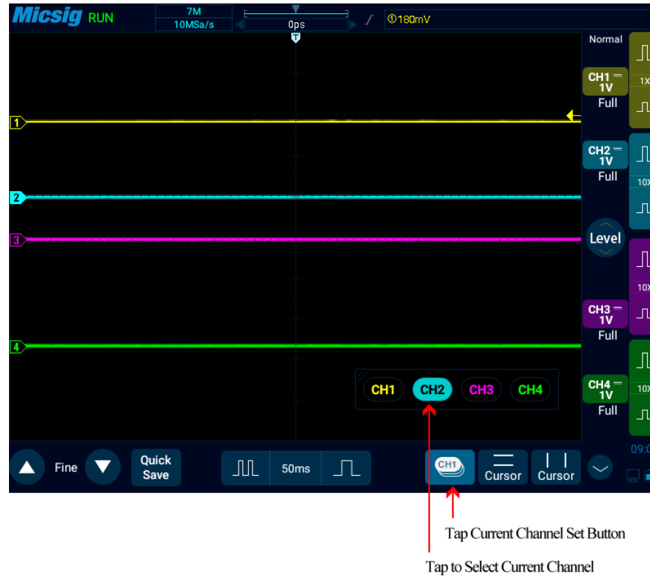
Figure 5-5 Using the Current Channel Selection Button
