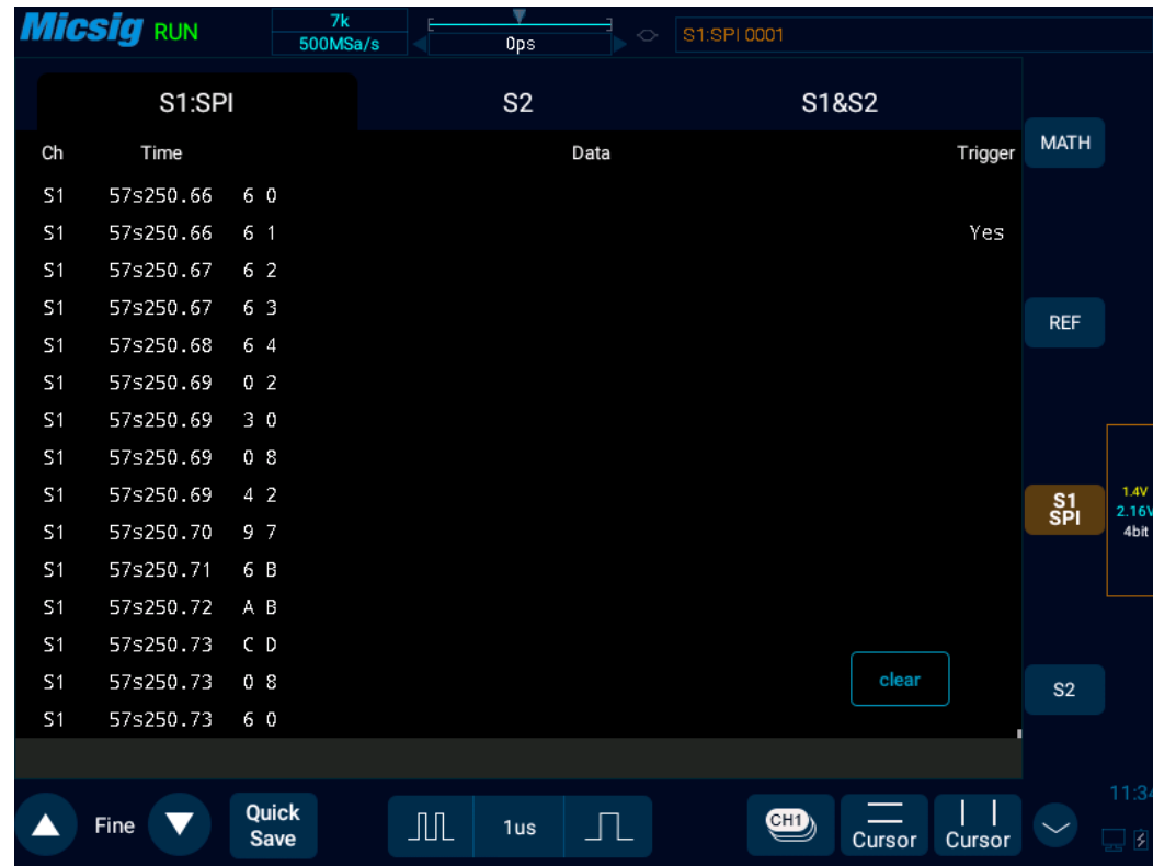
Figure 12-21 SPI Text Interface
