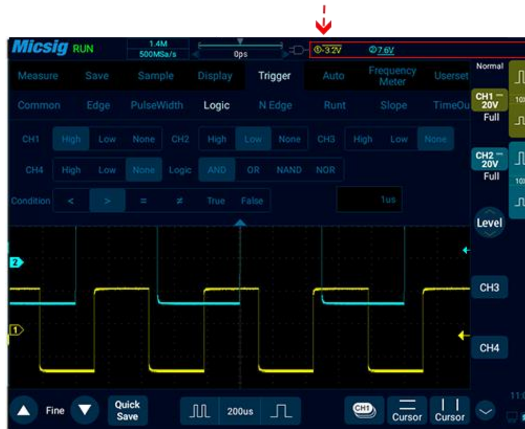
Figure 6-21 Trigger Level Adjustment
