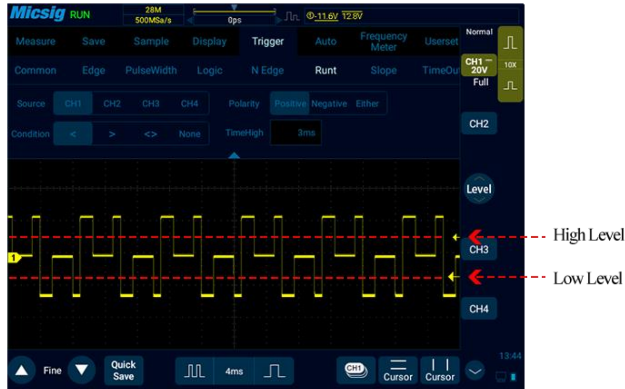
Figure 6-24 Runt Trigger Setting Menu
