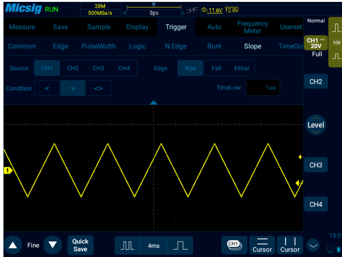
Figure 6-26 Slope Trigger Setting Menu
