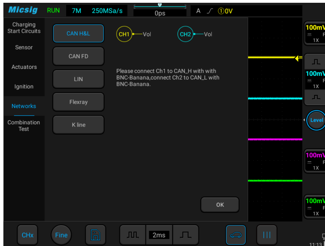
Figure 3-45 CAN BUS Test
