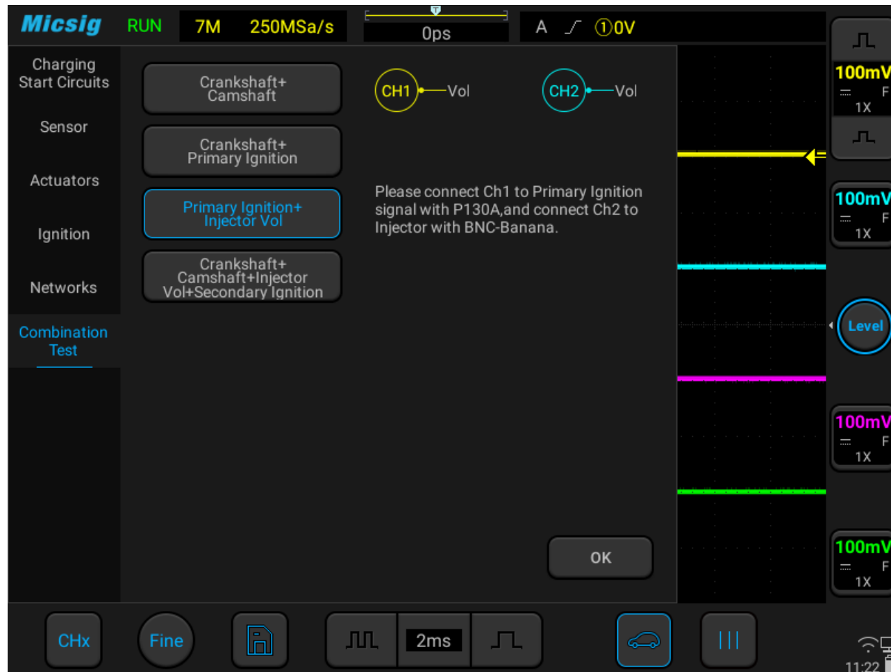
Figure 3-52 Primary ignition + Injector voltage
