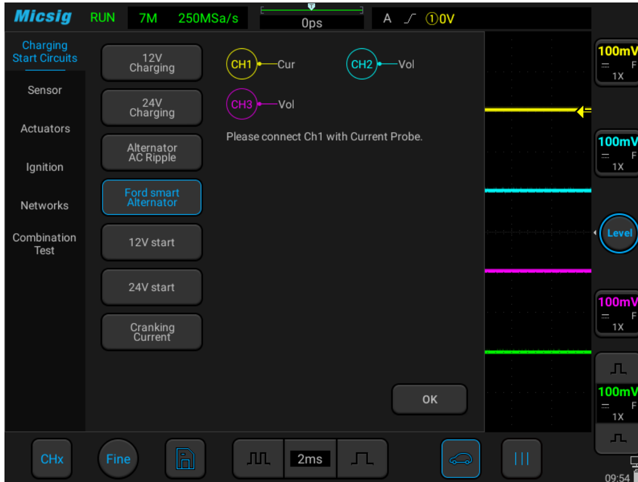
Figure 3-5 Ford Focus Smart Generator
