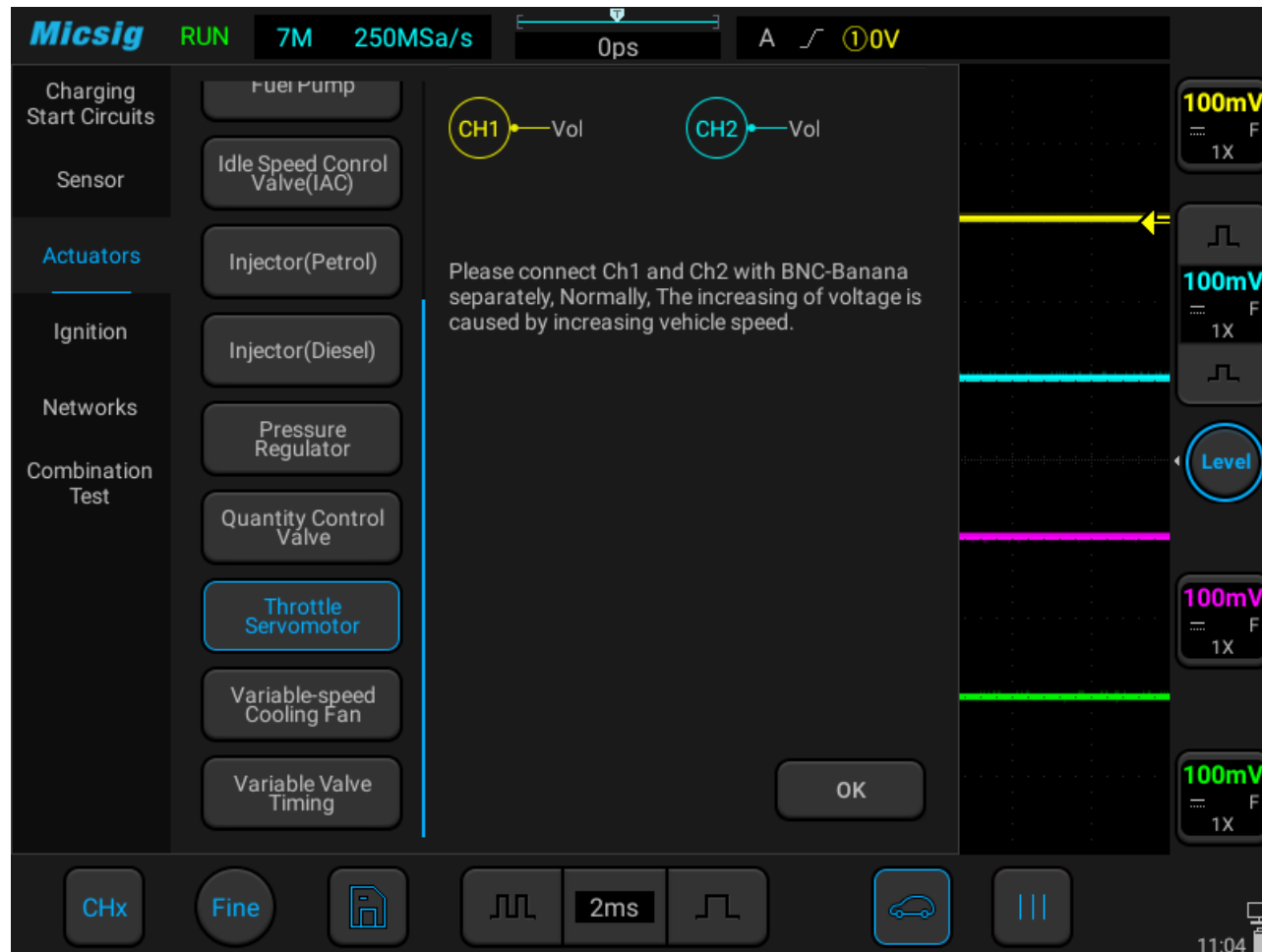
Figure 3-36 Throttle servo motor test
