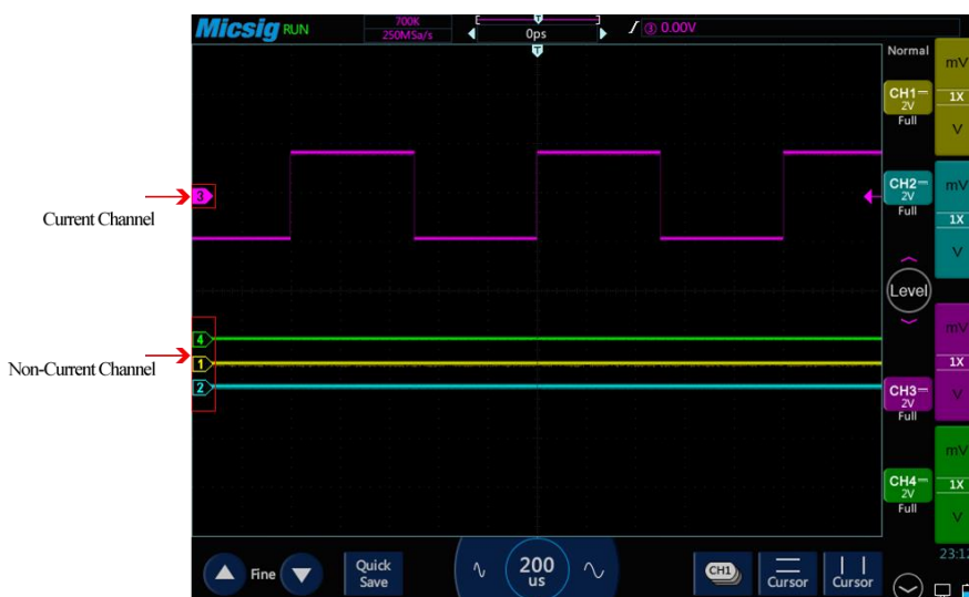
Figure 4-2 Current Channel and Non-Current Channel
