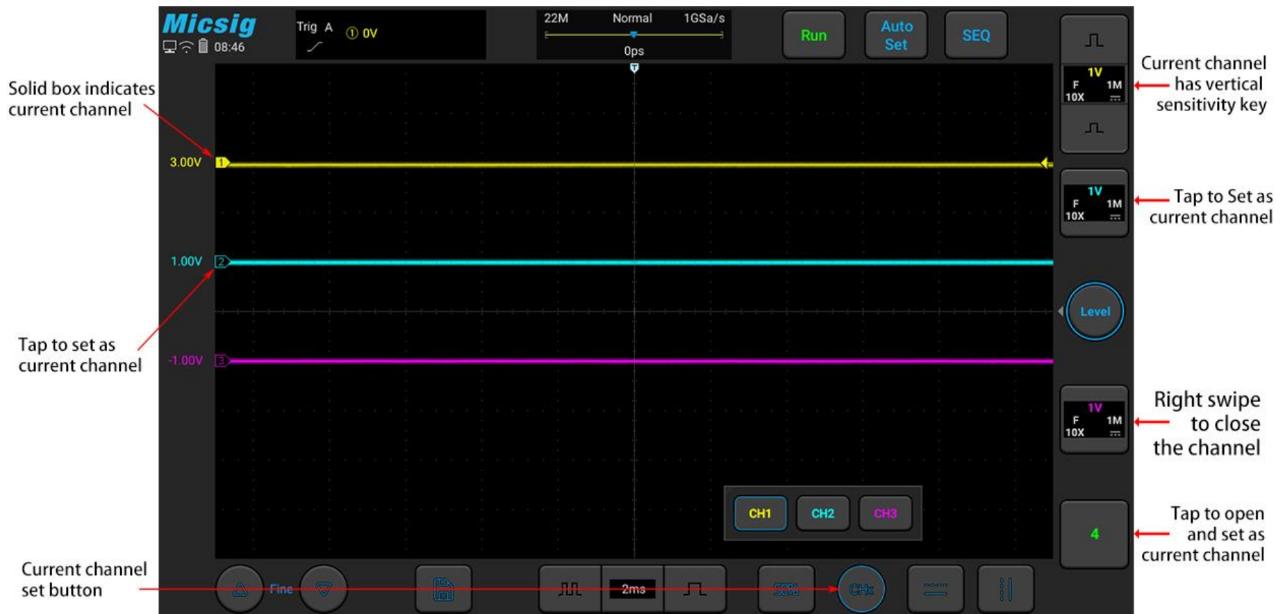
Figure 4-4 Channel Open, Close and Switching
