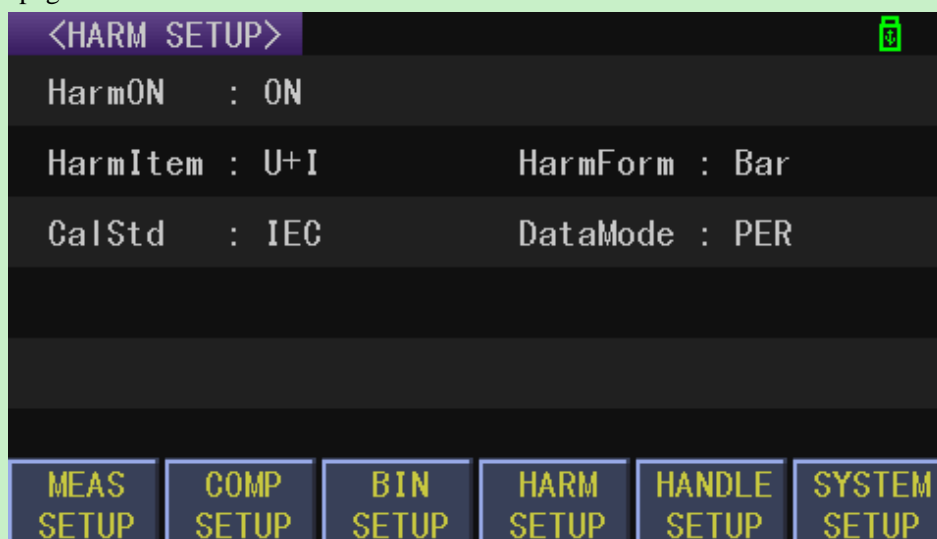
Figure 4-17 Harmonic setup interface
