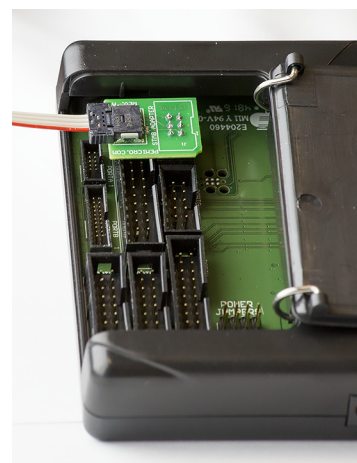
Figure 3-27: STM8 Adapter: 1) Bottom, 2) Top, 3) Connected To 6-Pin Header of Cyclone_Universal_FX (Adapter Sold Separately)
