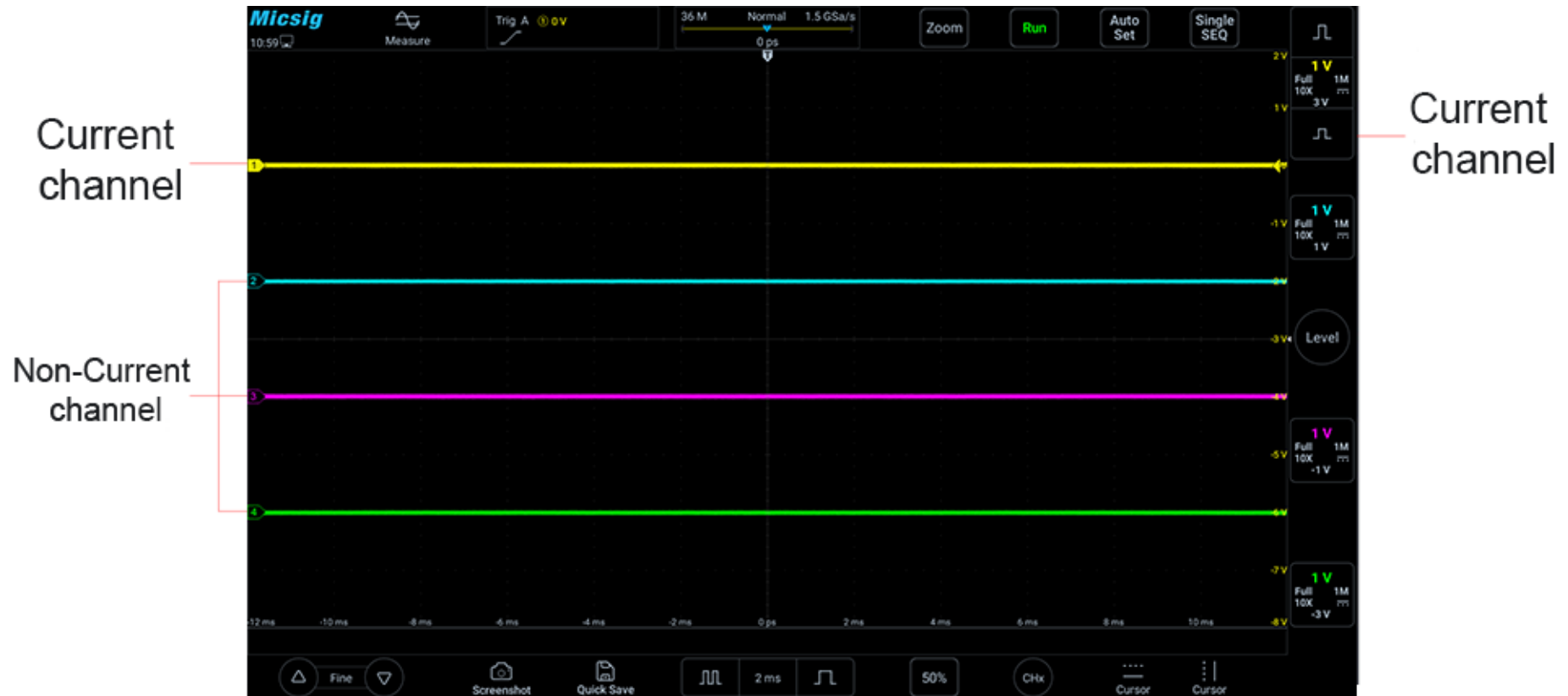
Figure 5-2 Current Channel and Non-Current Channel
