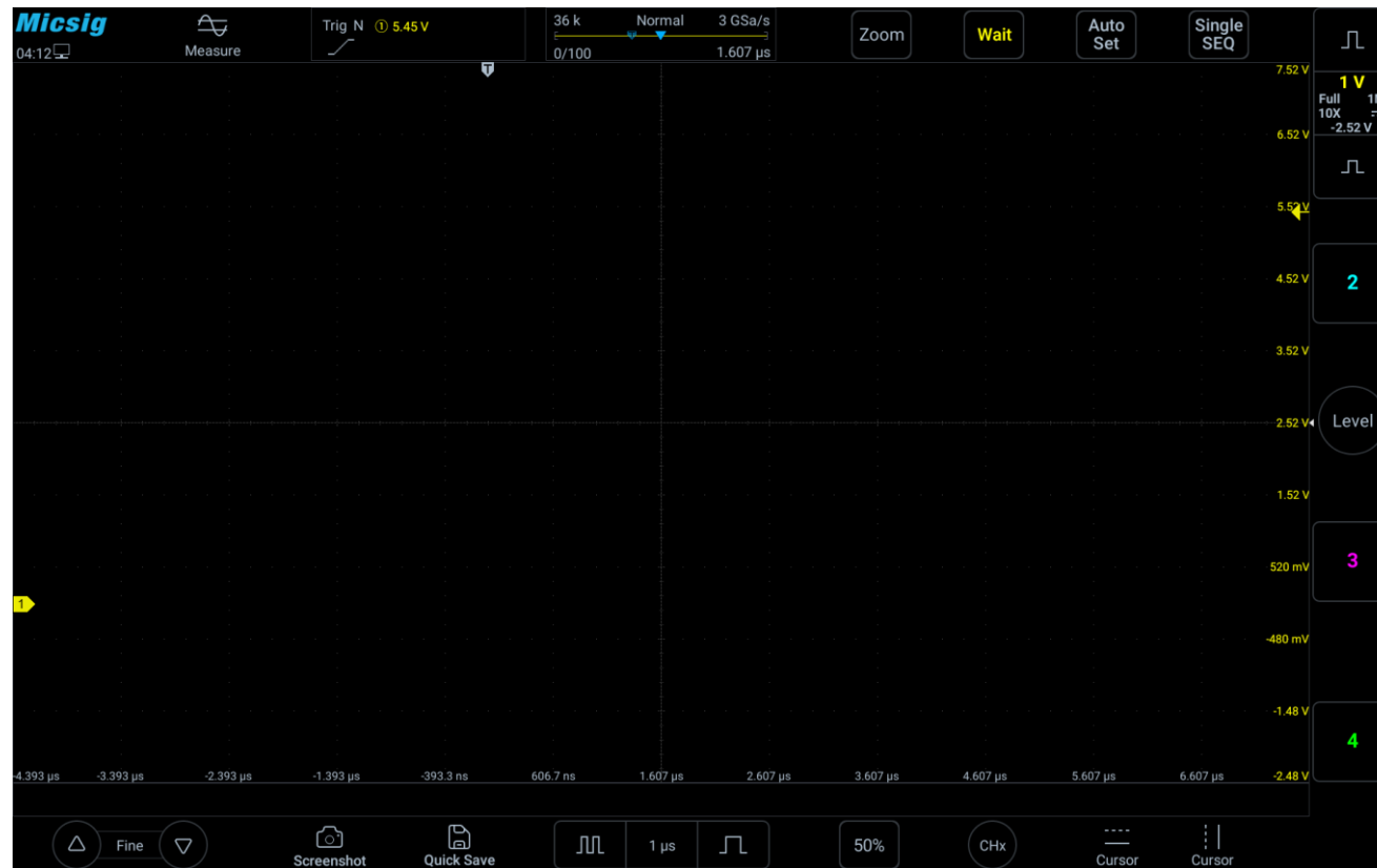
Figure 11-14 Single trigger segmented storage
