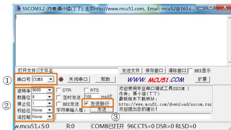
Figure 6-16 SSCOM3.2 Software Settings
